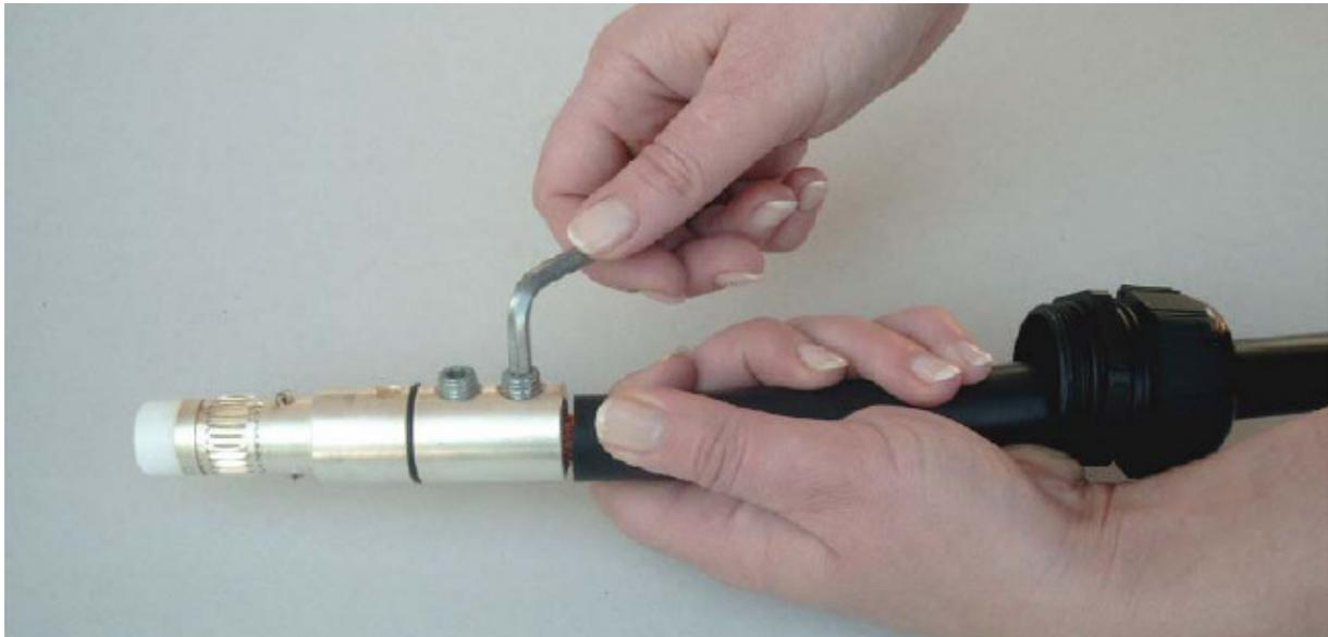
6. Fit the contact into the front insulator and visually align the Retention pin holes.
