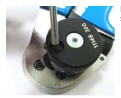
Place in the additional locator, straighten it and fix it by spinning.
