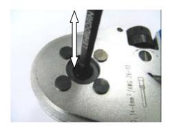
The **EPIC** CIRCON Crimp tool is fully opened. Spin the hand wheel until the scale shows  $\mathbf{2}$  and the hand wheel shows  $\mathbf{0}$ . Then close the EPIC CIRCON Crimp tool down to the end stop. In this set up the plug gauge  $\emptyset 2$  must be moveable with no scope between the crimp mandrels.
